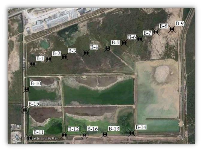
Figure 2.3 – Soil Borings Location Map (Showing Approximate Location)
