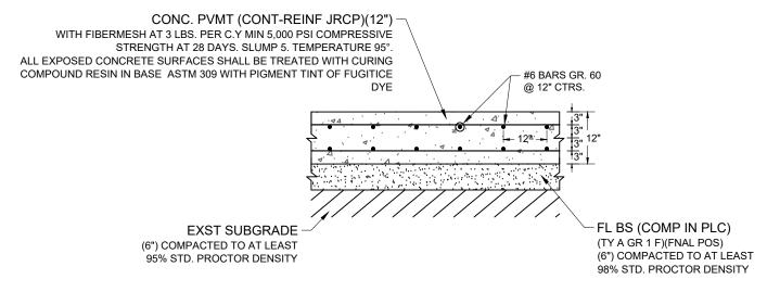
TYPICAL (12") CONCRETE PAVEMENT DETAIL
