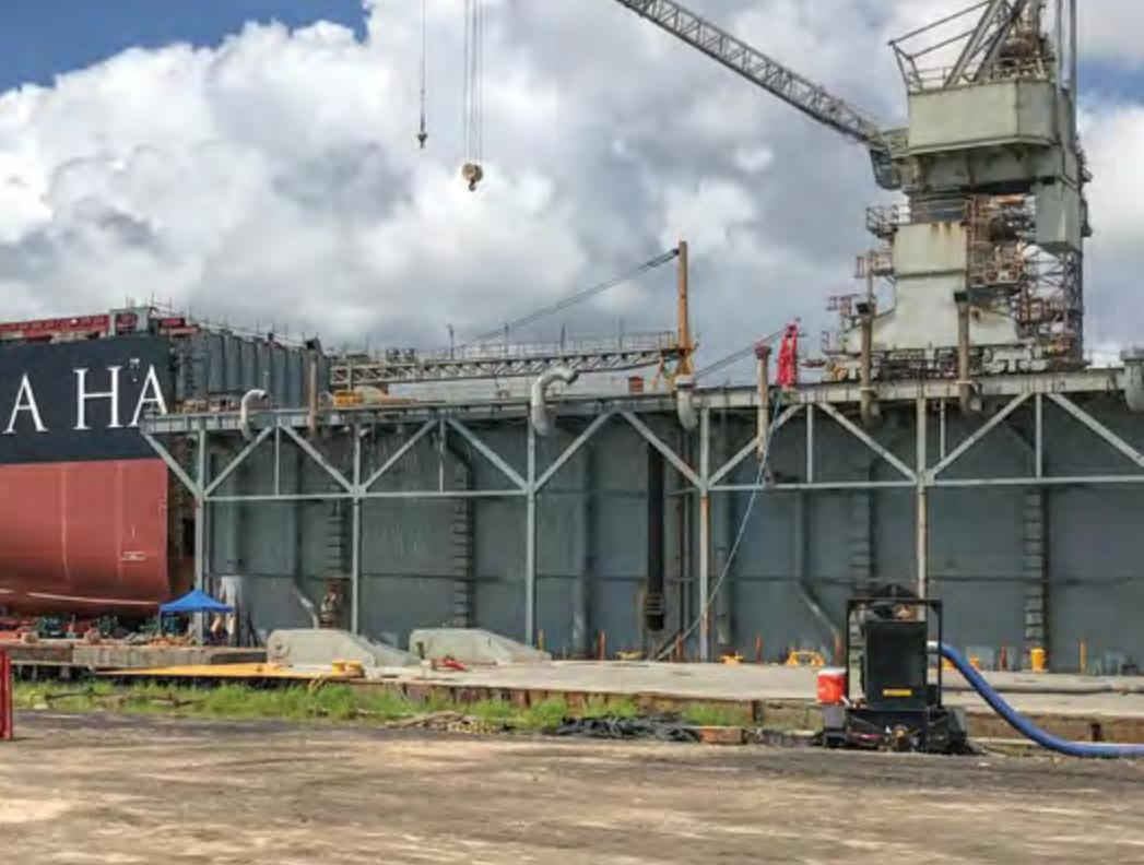
**Left:** The bow of the *M/V George III* is positioned onto a barge at Keppel AmFELS' yard. Delivery of the vessel to Pasha Hawaii is scheduled for summer 2020.
