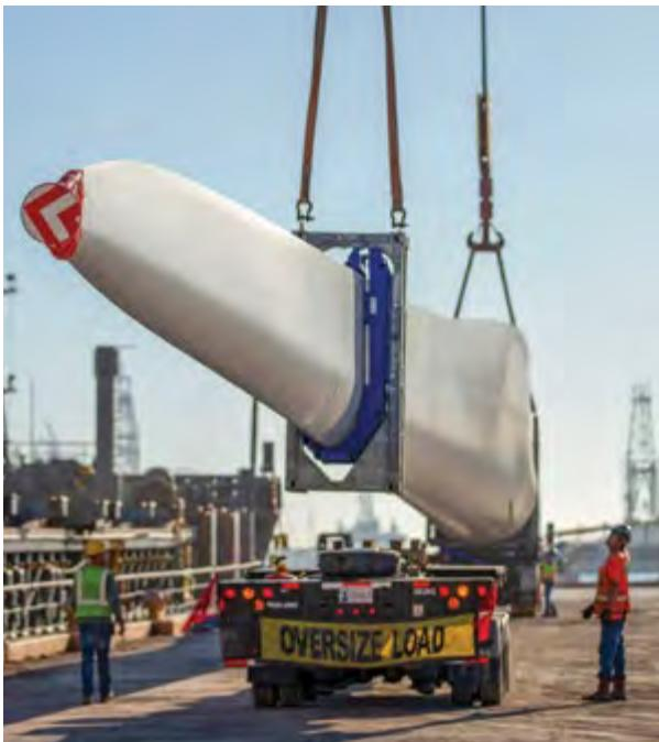
Windmill components are a common project cargo, with multiple and simultaneous providers utilizing the Port of Brownsville's expansive laydown assets.
